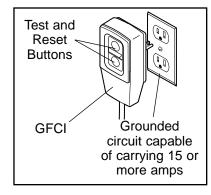
console (see USING THE CONSOLE on page 13). Once the unit is running, press the GFCI "test" button. The spa should shut off. Press the "reset" button. The spa should resume normal operation. If the spa continues to run after the "test" button is pressed, the GFCI is damaged. Do not use the spa until the GFCI has been repaired or replaced by a qualified electrician.
